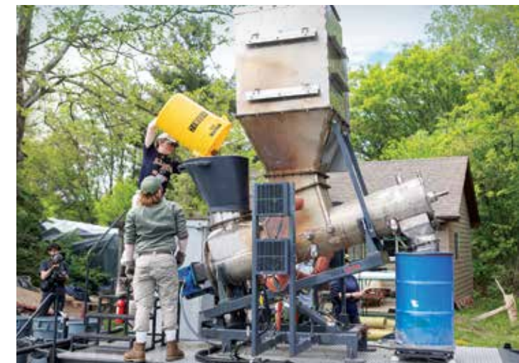
Students in the Professional Credentials and Training for Ecologists course learned to use equipment that converts organic matter into biochar. The charcoal-like substance is useful in ecological restoration projects.
